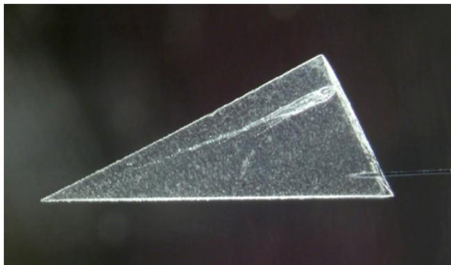
**Figure 3:** Track of a  $15\mu\text{m}$  cometary particle in aerogel, captured at  $6.1\text{ km/s}$  in the coma of Jupiter-family comet 81P/Wild 2 in January 2004. The Stardust cometary grain collection was much more numerous and easy to identify, contrary to the interstellar dust collection. Identification of faint and rare interstellar grain tracks needed a citizen science effort.
