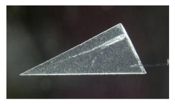
**Figure 3**: Track of a  $15\mu$ m cometary particle in aerogel, captured at 6.1 km/s in the coma of Jupiter-family comet 81P/Wild 2 in January 2004. The Stardust cometary grain collection was much more numerous and easy to identify, contrary to the interstellar dust collection. Identification of faint and rare interstellar grain tracks needed a citizen science effort.
