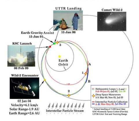
**Figure 1**: Besides collecting dust from comet Wild 2, the Stardust space probe exposed collectors to the interstellar dust stream from 22 Feb 2000 to 1 May 2000 and from 5 Aug 2002 to 9 Dec 2002 i.e. for a total of 195 days. Courtesy NASA/JPL-Caltech.
