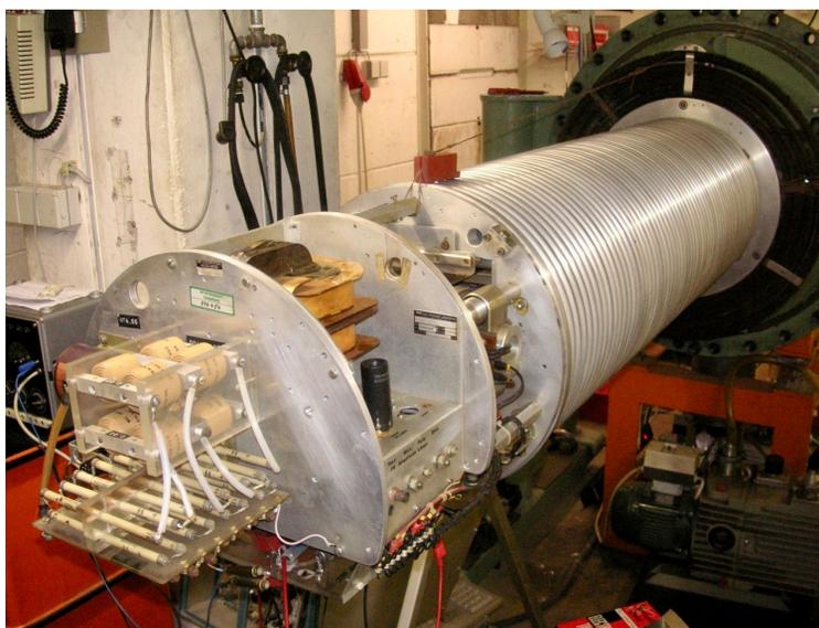
**Figure 5:** The Heidelberg dust accelerator can accelerate tiny particles up to 100 km per second using an acceleration voltage of 6 million volts. Particles shot on Aerogel served as calibration images for stardust@home searchers before finding interstellar dust particles.
