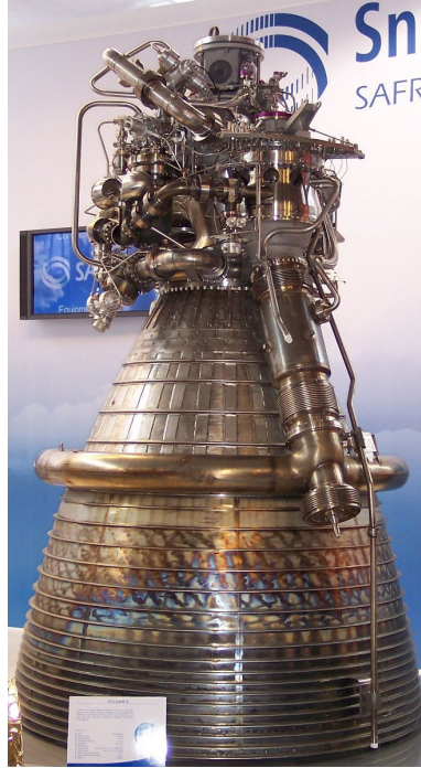
Figure 3.7 An example for a de Laval nozzle is the Vulcain-II engine of an Ariane 5 rocket (Wikipedia, Creative Commons License)
