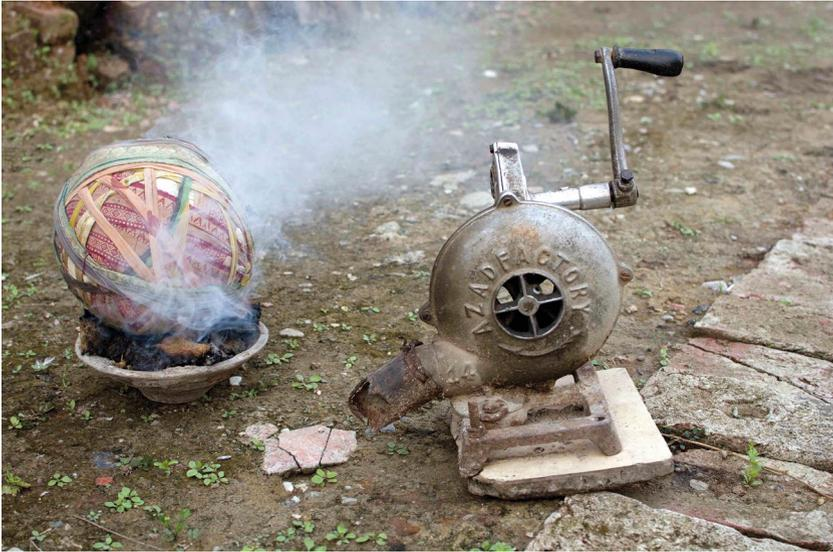
Figure 4: Pre-processed cinnabar is wrapped in a cotton ball (*kanduk*) and heated over a tray of cow dung with the help of a hand-operated bellows. It is then covered with a clay bowl and kept overnight, smoldering. Dehradun, 2013.
