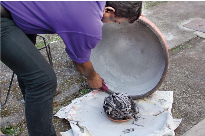
Figure 5: Balendu Prakash opens the *Kanduk Yantra* (a ball-like apparatus to distill mercury from cinnabar) the next morning; the wrapped-up pre-processed cinnabar had smoldered inside the cotton ball all night. Dehradun, 2013.
