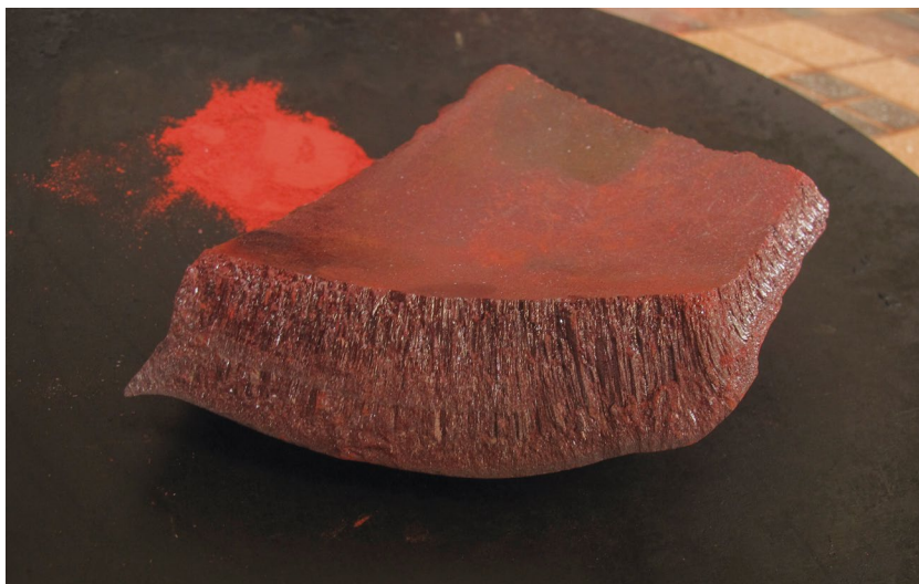
Figure 34: A piece of artificial cinnabar before grinding (right) and ground up powdered cinnabar (left). Photo by author (Gerke 2015/CC-BY-SA 4.0).
