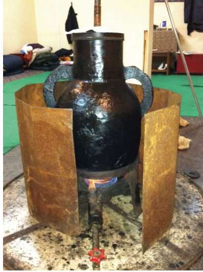
Figure 19: Since 1982, the same caldron has been used to boil mercury, and since 1987, a gas stove to better regulate the heat. The shield around it protects the gas flame from air currents. Photo: Men-Tsee-Khang (Men-Tsee-Khang 2011 / CC-BY-SA 4.0).
