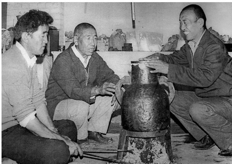
Figure 18: The metal caldron made especially to boil mercury. Lamempa Tenzin Chödrak (right) sealing the caldron, with Lamempa Jamyang Tashi (middle) and Dr. Tendzin Namgyel (left), Thekchen Chöling, 1982. Photo: Men-Tsee-Khang (Men-Tsee-Khang 1982 / CC-BY-SA 4.0).
