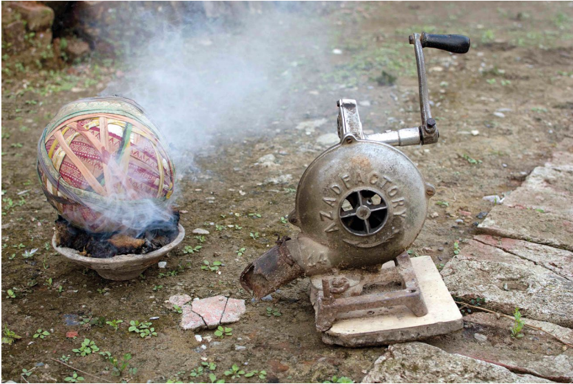
Figure 4: Pre-processed cinnabar is wrapped in a cotton ball ( kanduk ) and heated over a tray of cow dung with the help of a hand-operated bellows. It is then covered with a clay bowl and kept overnight, smoldering. Dehradun, 2013. Photo: Thomas K. Shor (Shor 2013 / CC-BY-SA 4.0).
