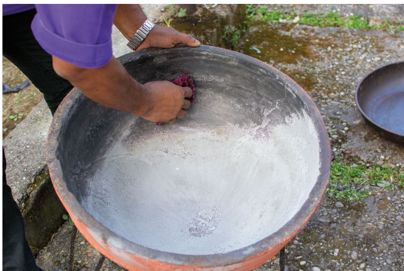
Figure 6: Mercury pellets form and collect at the bottom of the earthen bowl as Balendu Prakash scrapes the evaporated mercury dust off the sides. Dehradun, 2013. Photo: Thomas K. Shor (Shor 2013/CC-BY-SA 4.0).
