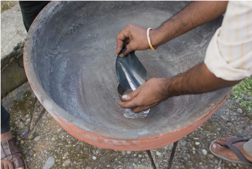
Figure 8: The distilled mercury is collected and further filtered and processed before use. Dehradun, 2013. Photo: Thomas K. Shor (Shor 2013/CC-BY-SA 4.0).
