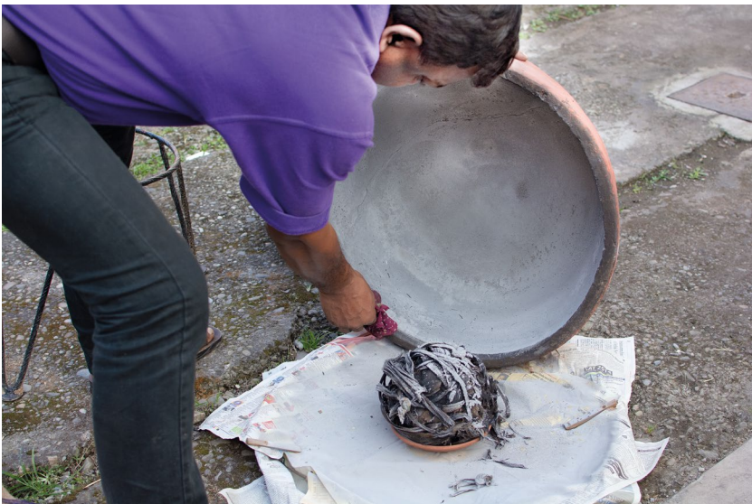
Figure 5: Balendu Prakash opens the Kanduk Yantra (a ball-like apparatus to distill mercury from cinnabar) the next morning; the wrapped-up pre-processed cinnabar had smoldered inside the cotton ball all night. Dehradun, 2013. Photo: Thomas K. Shor (Shor 2013 / CC-BY-SA 4.0).
