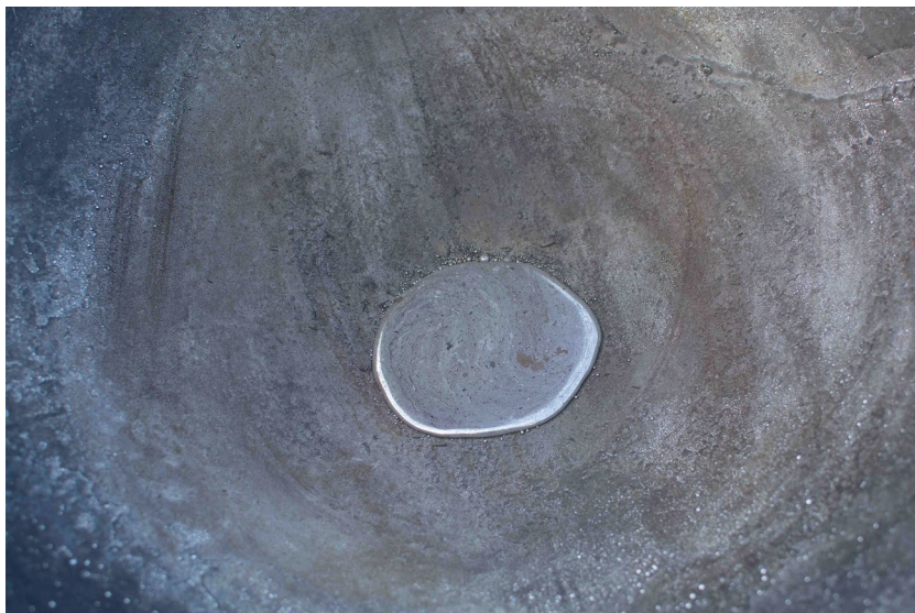
Figure 7: The amount of mercury distilled through the Kanduk Yantra. Dehradun, 2013. This method extracts about 700 grams of mercury from one kilogram of mercury sulfide ore (Prakash 2013, 212). Photo: Thomas K. Shor (Shor 2013/CC-BY-SA 4.0).
