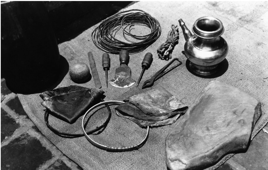
Fig. 338: Drum-maker's tools and raw material for making a nāykhī drum,
