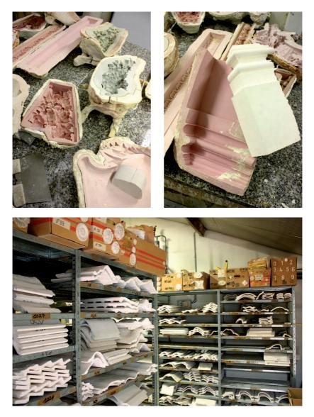
Figs. 1-3: The modern production process of plaster casts of/for decorative elements (above) and of/for architectural surfaces (below) and the storage of lightweight decorative elements (French: staff), photos taken at Maison Auberlet, successor of the original Auberlet et Laurent which executed the decoration of the 1:1-scale model of Angkor Wat at the International Colonial Exhibition in Paris 1931. Source: Michael Falser 5.2010
